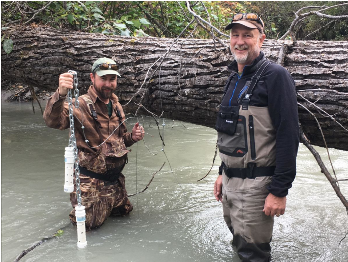
TWC Executive Director Derek Poinsette along with Richard Chapell, ADF&G Fishery Biologist (and TWC Board Member) install sensors at our newest water temperature monitoring site in the Tahini River.
