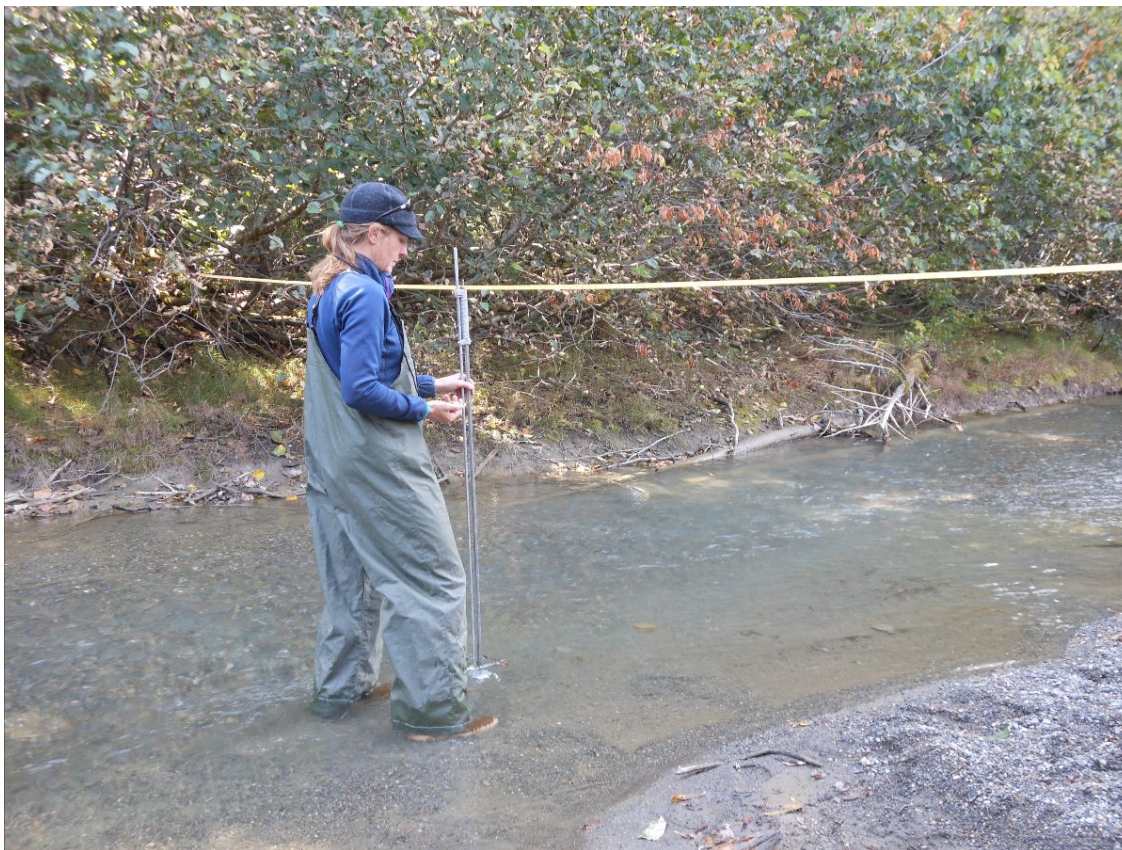
TWC Development Director Jenn Hamblen uses a flow meter to measure water velocity in Sarah Creek. The series of cross-sectional measurements of depth and velocity are used to calculate the total instantaneous discharge of the stream.
