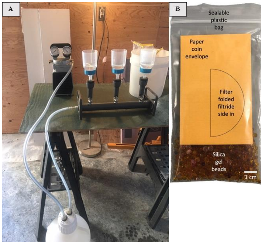
Figure 3: A: eDNA filtration set up. B: eDNA filter preservation with silica beads.
